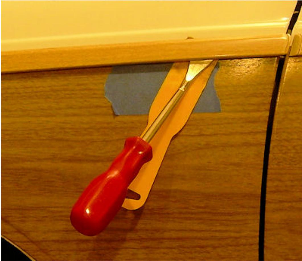
Once you get a couple of the clips popped loose, the molding will want to flop around a little bit. Use some masking tape to keep it in place until you get all the clips loose.
