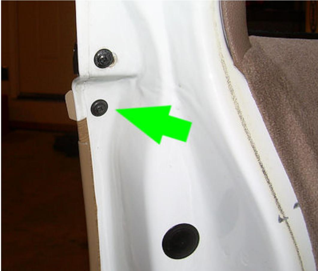
It also comes off the same way as the front fender molding once the screws are removed.
