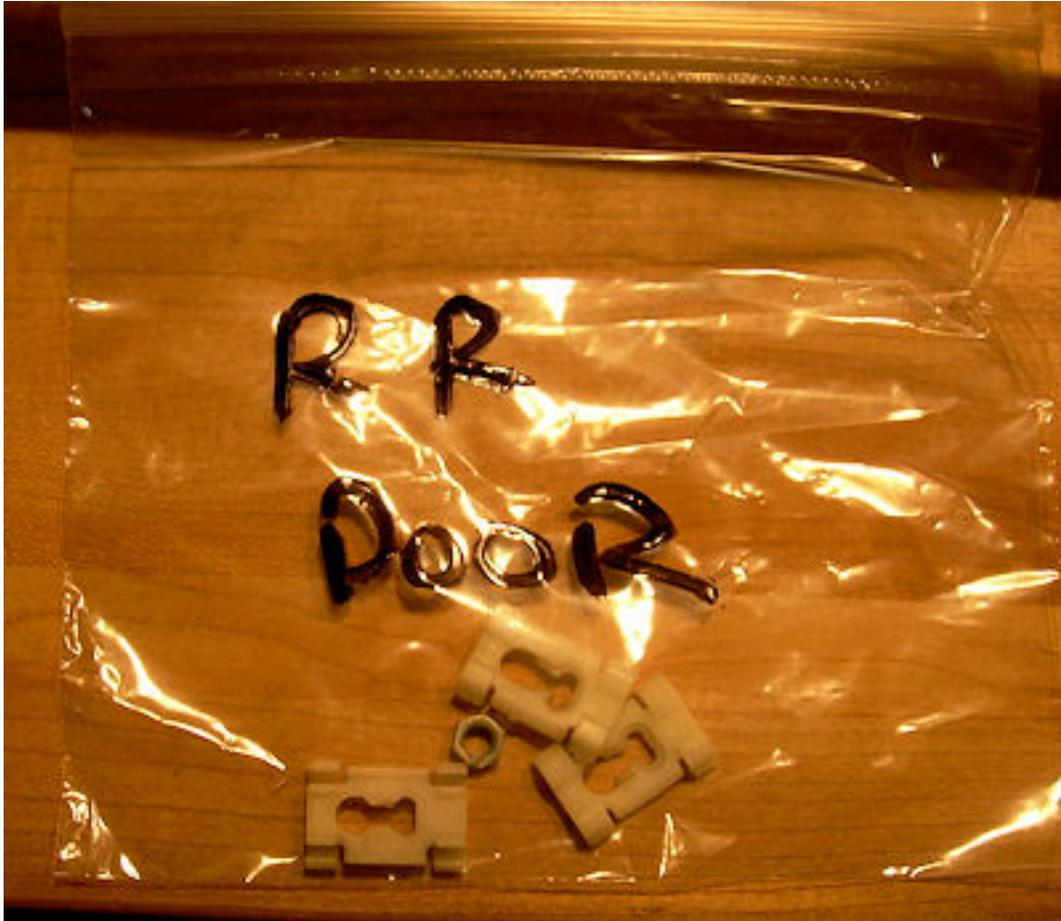
All the moldings are held on by clips. With the PRT and a little pressure, you'll be able to pop the moldings loose. So here we go. The first molding to come off is the molding that runs along the top of the fender. To find the clips, insert the plastic putty knife between the molding and the sheet metal, and then move it in any direction until you run into resistance. When you run into resistance, you are close to one of the clips.
